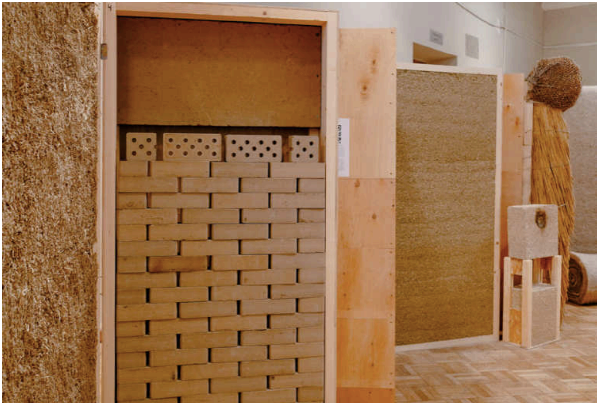
The photo shows eco-friendly bricks made of natural clay by the Ukrainian brand Glinko. Photo: Natalia Azarkina
