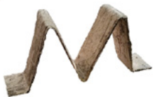
Fig. 14: Load-bearing capacity of wool-clay-jute mixtures © Leon Zimmermann / Institute for Architecture-Related Art, TU Braunschweig
