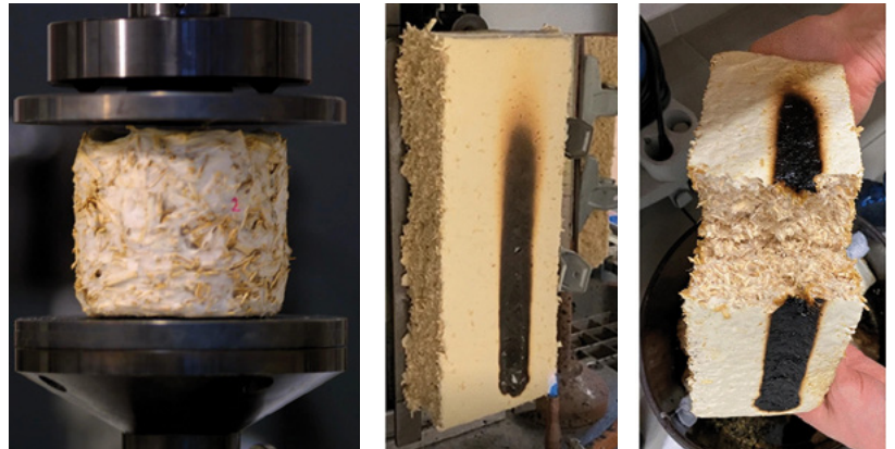
Fig. 7: Fire tests according to EU standards showing that only the outer layer of the mycelium burns, while the inner part remains unaffected. © Pohl et al. (2022) Fungal Biol Biotechnol 9 | Schmidt et al. (2023) Fungal Biol Biotechnol 10
