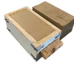
Fig. 25: Clay brick in formwork and switched off © Leon Zimmermann / Institute for Building Construction, TU Braunschweig
