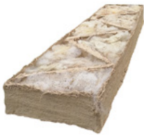
Fig. 23: Building block made of clay-jute folded and insulated with raw wool © Leon Zimmermann / Institute for Architecture-Related Art, TU Braunschweig
