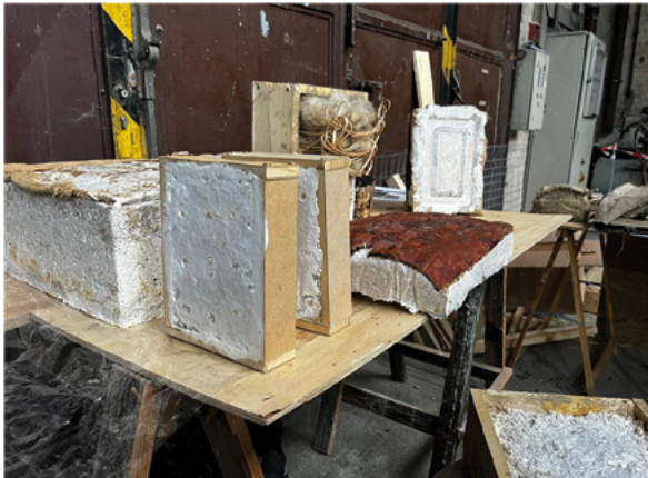
Fig. 18, 19: Samples for measuring how well a material conducts heat, ZNE! Berlin 2023 and TU Braunschweig © IBEA, Tobias Pörschke
