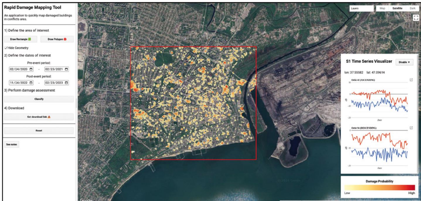
Fig. 15: Prototype dashboard of the Rapid Damage Mapping Tool, showing damage estimates for a region in Mariupol and visualization of the Sentinel-1 time series. (Source: O. Dietrich et al. 2025, ETH Zürich); https://arxiv.org/pdf/2406.02506
