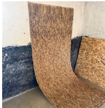
Fig. 25: Flexible reed board, strong, malleable, versatile
