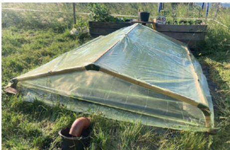
Fig. 26–28: Garden biogas plant © (B)energy
