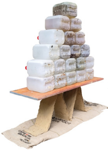
Fig. 20: Load test of a wool-clay-jute fold with over 230 kg © Leon Zimmermann / Institute for Architecture-Related Art, TU Braunschweig
