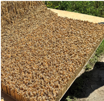
Fig. 24: Natural reed board, ecological and heat insulating
