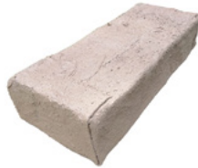
Fig. 24: Finished clay insulation block © Leon Zimmermann / Institute for Architecture-Related Art, TU Braunschweig
